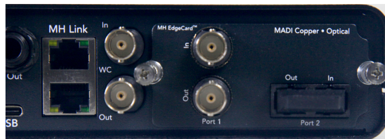
Figure 1.4: Insert EdgeCard into Slot
