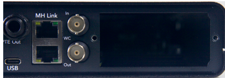
Figure 1.3: Remove Cover Plate
